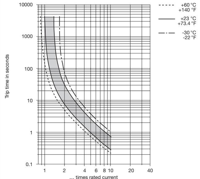
The time/current characteristic curve depends on the ambient temperature prevailing. In order to eliminate nuisance tripping, please multiply the circuit breaker current ratings by the derating factor shown below. See also section 9 – Technical information.
