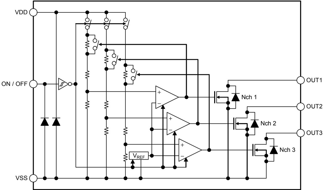
**Remark** Diodes in the figure are parasitic diodes.
