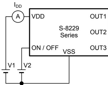
Figure 6 Test Circuit 2
