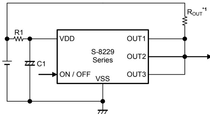
\*1. Set up  $R_{OUT}$  as 220  $\Omega$  or more so that the power dissipation is not exceeded.
