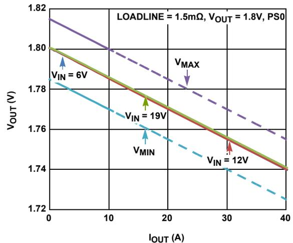
FIGURE 2. LOAD LINE REGULATION
