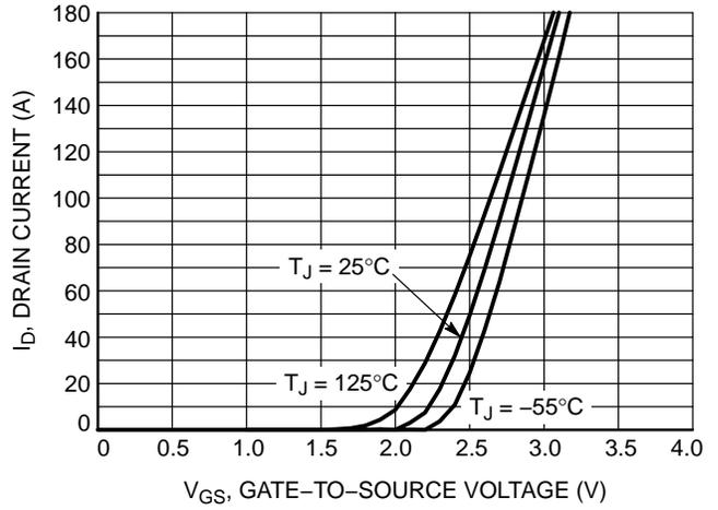
Figure 2. Transfer Characteristics
