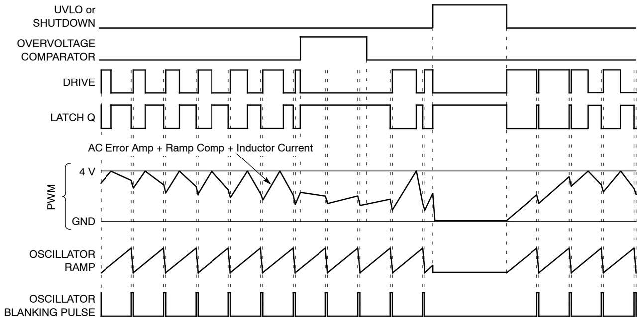
Figure 2. Timing Diagram
