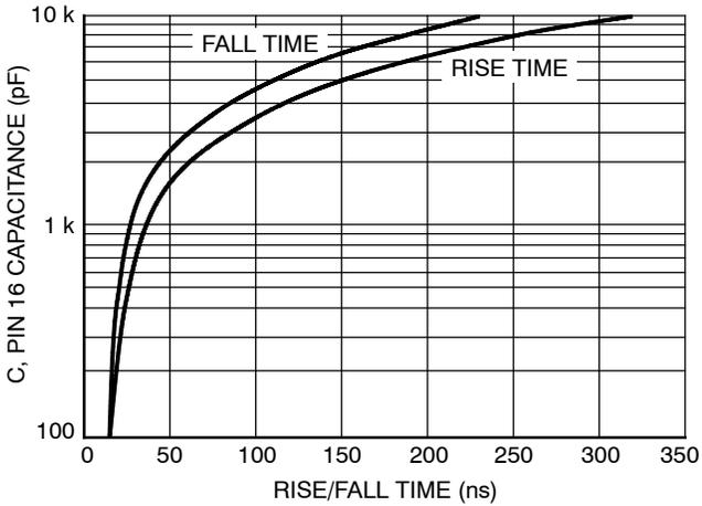
**Figure 18. Capacitance versus 10-90% Drive Rise and Fall Times**
