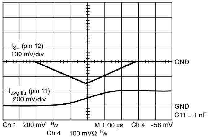
Figure 15. Current Sense Amplifier High Frequency Response
