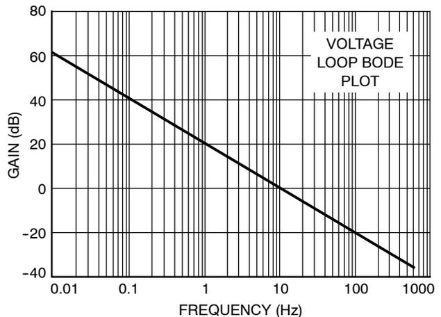
**Figure 44. Open Loop Gain of Voltage Loop**
