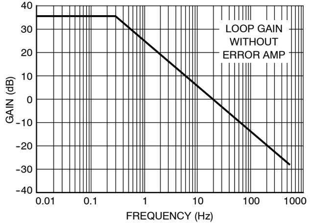
**Figure 43. Open Loop Gain Less Error Amp**
