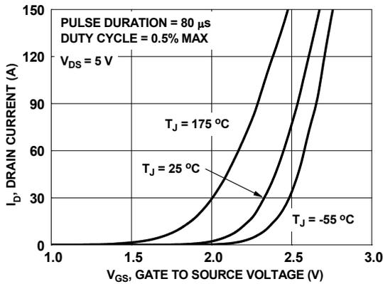
Figure 5. Transfer Characteristics
