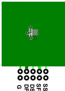
a.  $53\text{ }^\circ\text{C/W}$  when mounted on a 1 in<sup>2</sup> pad of 2 oz copper.
