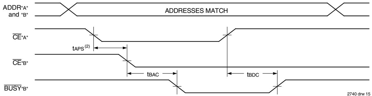
Waveform of **BUSY** Arbitration Cycle Controlled by Address Match Timing<sup>(1)</sup> ( $M/\bar{S} = V_{IH}$ )
