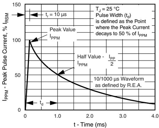
Fig. 3 - Pulse Waveform
