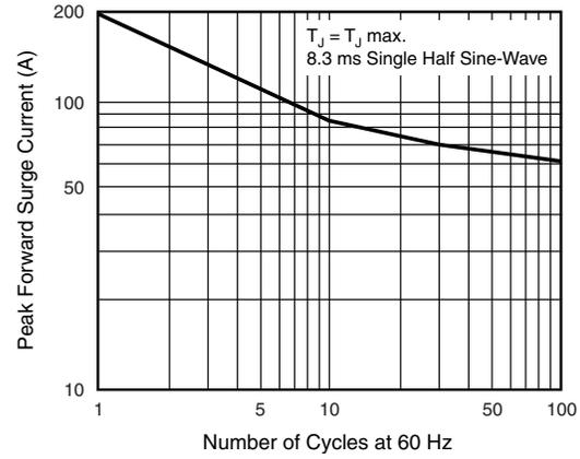
Fig. 5 - Maximum Non-Repetitive/Peak Forward Surge Current
