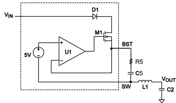
**Figure 3: Internal Bootstrap Charging Circuit Startup and Shutdown**
