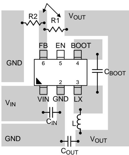
LX should be connected to inductor by wide and short trace, and keep sensitive components away from this trace.
