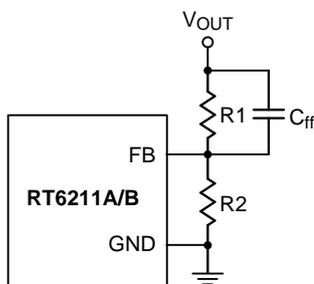
Figure 1. C<sub>ff</sub> Capacitor Setting
