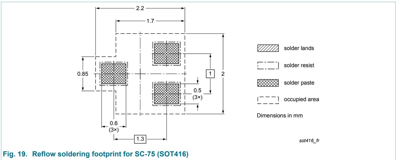
Fig. 19. Reflow soldering footprint for SC-75 (SOT416)
