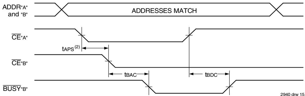
Waveform of **BUSY** Arbitration Cycle Controlled by Address Match Timing<sup>(1)</sup> ( $M/\bar{S} = V_{IH}$ )
