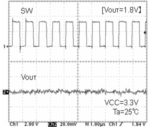
Fig.15 SW waveform I<sub>o</sub>=10mA
