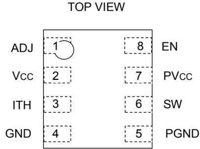
Fig.2 Pin Configuration
