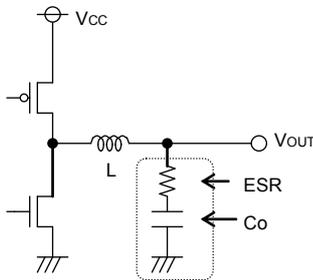
Fig.27 Output capacitor
