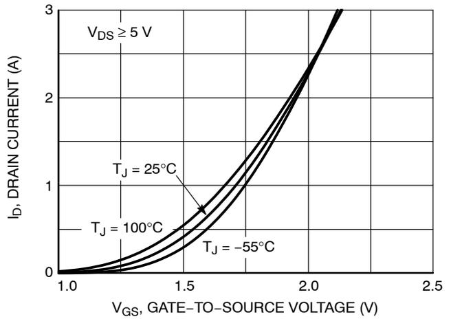
Figure 2. Transfer Characteristics
