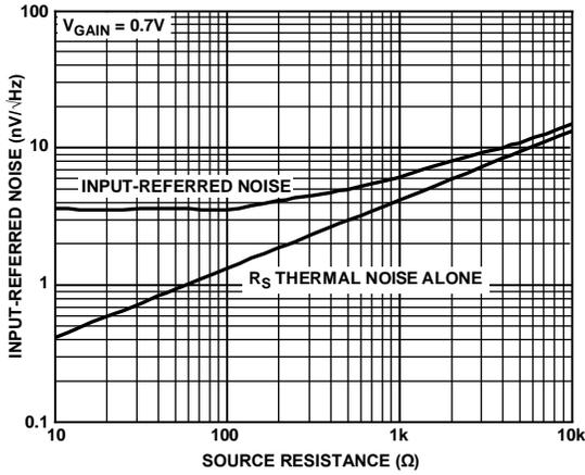
Figure 33. Input-Referred Noise vs. Source Resistance (See Figure 72)
