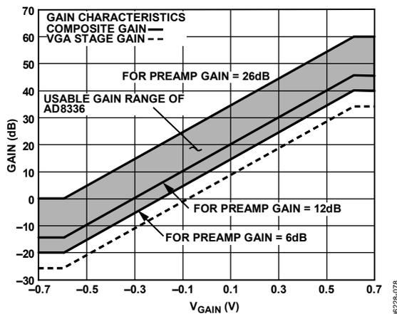
Figure 78. Ideal Gain Characteristics of the AD8336
