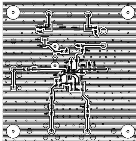
Figure 83. Component Side Copper
