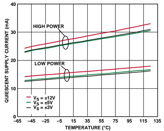
Figure 55. I<sub>Q</sub> vs. Temperature for Three Values of Supply Voltage and High and Low Power (See Figure 68)
