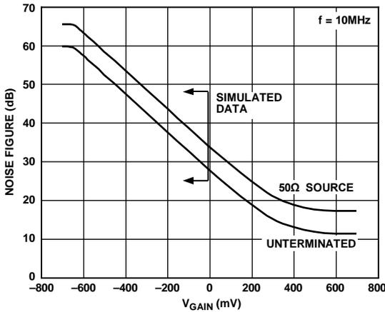
Figure 34. Noise Figure vs.  $V_{GAIN}$  (See Figure 63)
