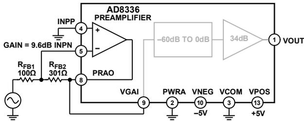
Figure 81. Circuit Configuration for Inverting Gain
