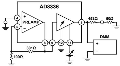
Figure 60. Offset Voltage
