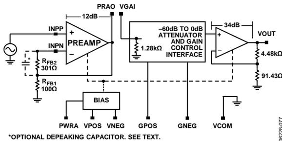
Figure 77. Simplified Block Diagram
