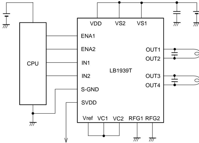
Constant voltage control mode: OUT outputs a 1.75 V, which is  $V_{ref} (0.9 \text{ V}) \times 1.95$ .
