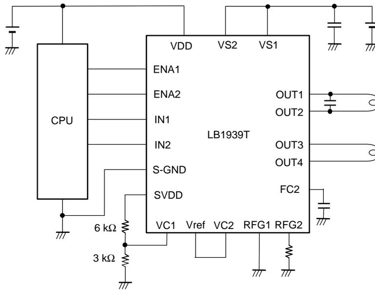
Channel 1 operates in constant voltage control mode: OUT outputs  $V_{DD} \times 3K/(3K + 6K) \times 1.95$
