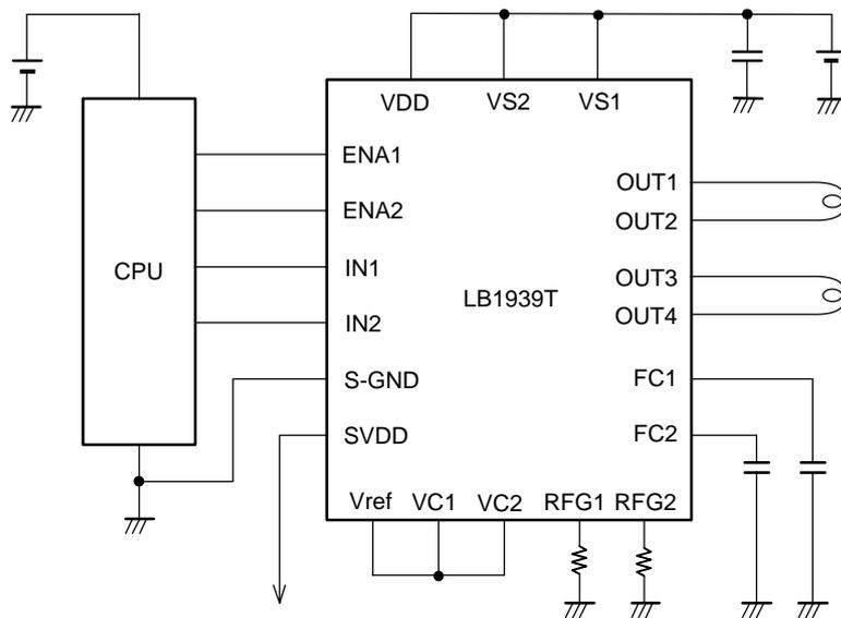
Constant current control mode: The RFG voltage is controlled so that  $V_{ref}/4.5 = 0.2 \text{ V}$ .
