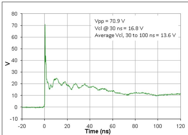
Figure 1. ESD Clamping Voltage Screenshot
