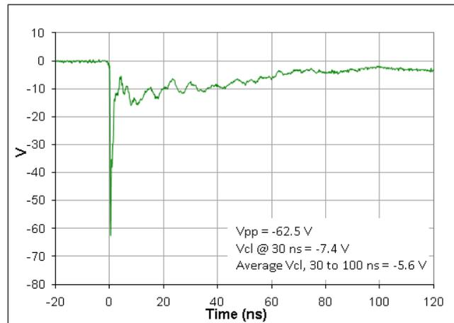
Figure 2. ESD Clamping Voltage Screenshot
