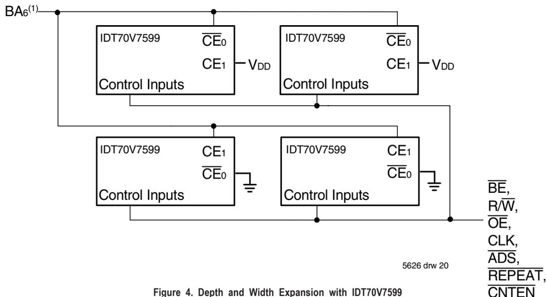
Figure 4. Depth and Width Expansion with IDT70V7599
