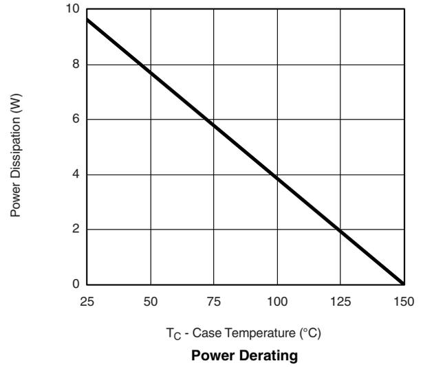
\* The power dissipation  $P_D$  is based on  $T_{J(max)} = 175\text{ °C}$ , using junction-to-case thermal resistance, and is more useful in settling the upper dissipation limit for cases where additional heatsinking is used. It is used to determine the current rating, when this rating falls below the package limit.
