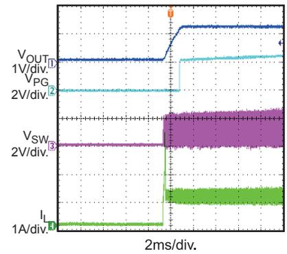
**VIN Shutdown (PG) with 1A Load**
