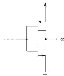
Figure 3-5:  $\overline{CD}$  Circuit
