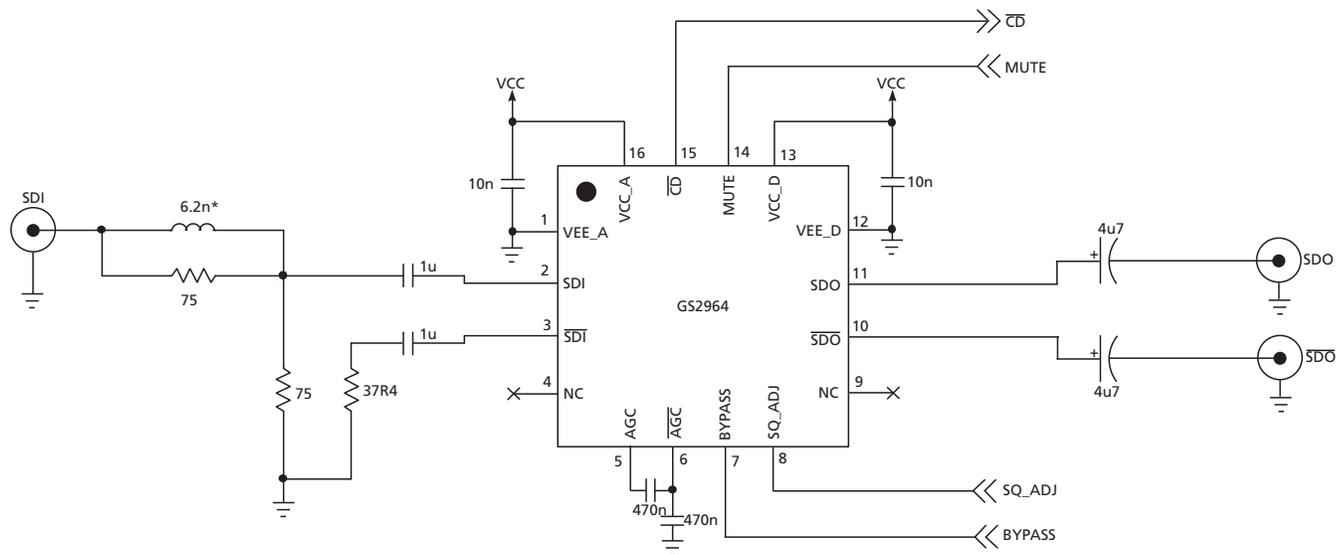
NOTE: All resistors in Ohms, capacitors in Farads, and inductors in Henrys, unless otherwise noted.
