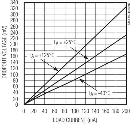
**DROPOUT VOLTAGE vs. LOAD CURRENT (OUTPUT = 5V)**
