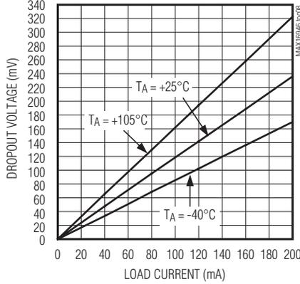
**DROPOUT VOLTAGE vs. LOAD CURRENT (OUTPUT = 8.5V)**
