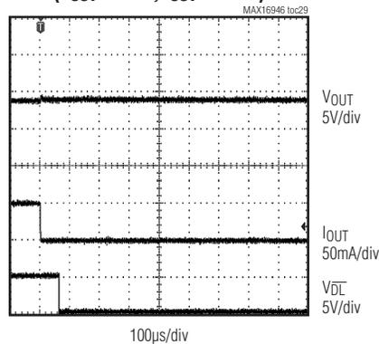
**CLEARING OPEN-LOAD FAULT
