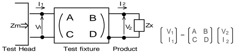
(2) The impedance of chip coil  $Z_x$  and measured value  $Z_m$  can be described by input/output current/voltage.
