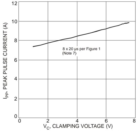
Fig. 4 Clamping Voltage vs. Peak Pulse Current
