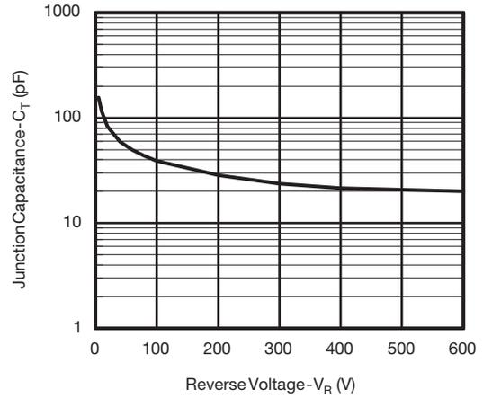
Fig. 3 - Typical Junction Capacitance vs. Reverse Voltage
