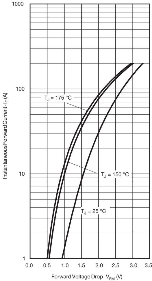
Fig. 1 - Typical Forward Voltage Drop Characteristics
