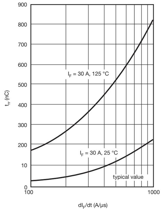
Fig. 8 - Typical Stored Charge vs.  $di_F/dt$
