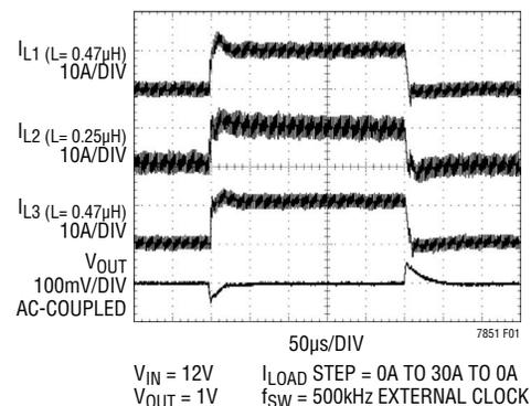
Figure 1. Mismatched Inductor Load Step Transient Response
