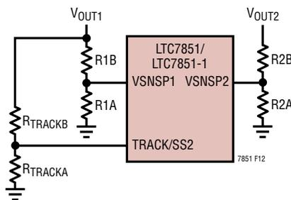
Figure 13. Output Voltage Tracking Using the TRACK/SS Pin
