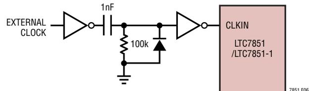
Figure 6. The Circuit to Keep the CLKIN Pin High Before the External Clock Starts Switching
