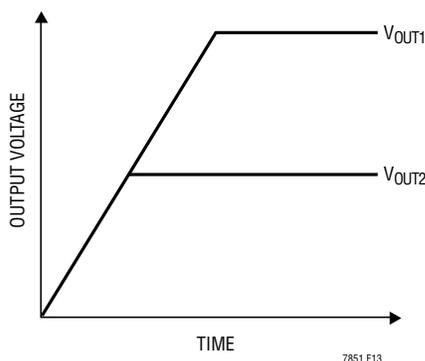
Figure 14. Coincident Tracking
