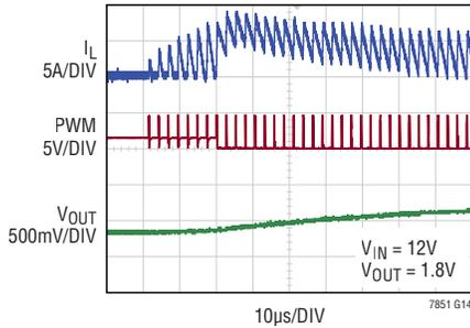
**Start-Up Response Into a 300mV Prebiased Output (Single Phase Using FDMF5820DC DrMOS)**
