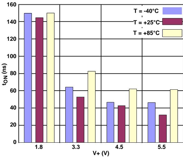
FIGURE 16. TURN - ON TIME vs SUPPLY VOLTAGE
