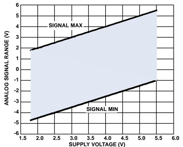
FIGURE 13. ANALOG SIGNAL RANGE vs SUPPLY VOLTAGE
