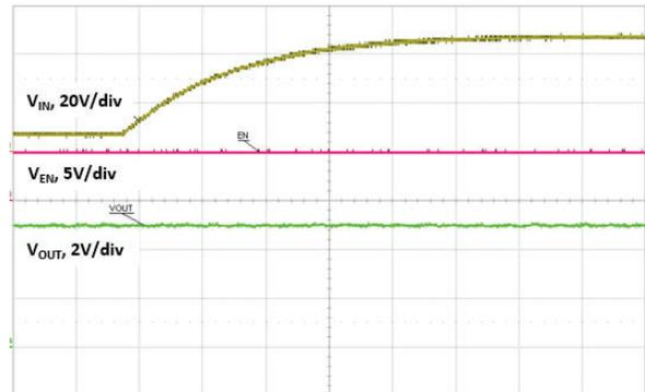
Fig. 26 - Line Transient (8 V to 48 V), Time = 10 ms/div
