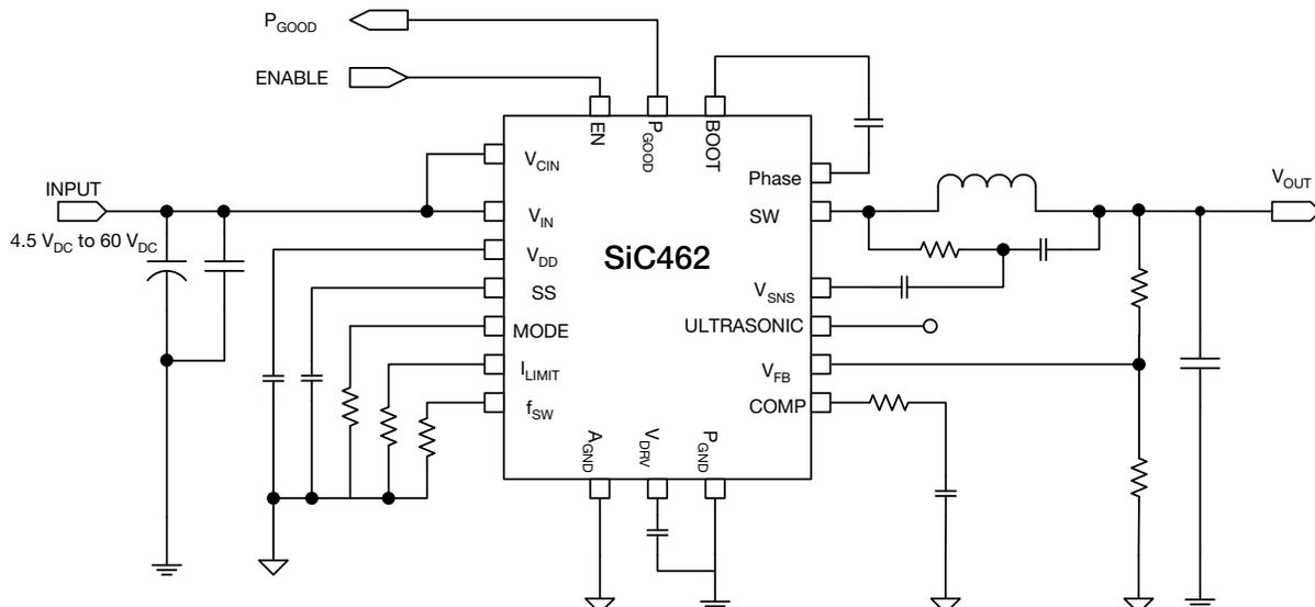
Fig. 1 - Typical Application Circuit for SiC462
