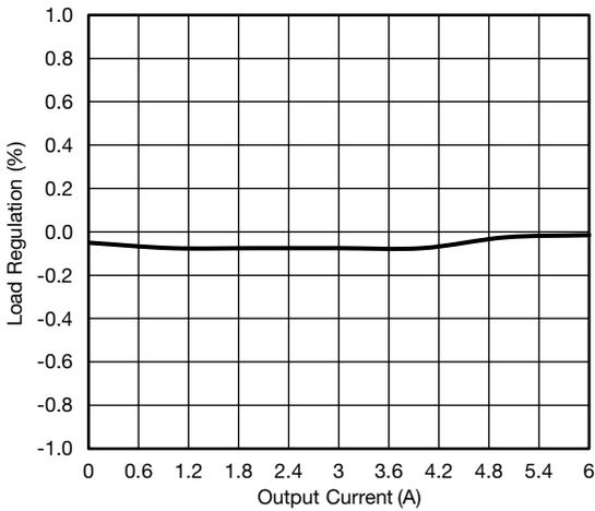
**Fig. 17 - Load Regulation,  $V_{OUT} = 12\text{ V}$**
