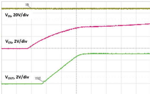
Fig. 23 - Start-Up with EN, Time = 1 ms/div
