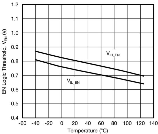
**Fig. 18 - EN Logic Threshold vs. Junction Temperature**
