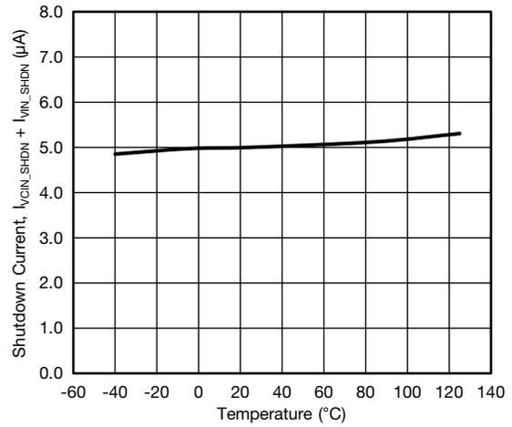
**Fig. 19 - Shutdown Current vs. Junction Temperature**
