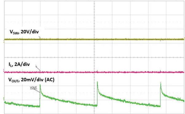
**Fig. 29 - Output Ripple PSM, Time = 10 ms/div**
