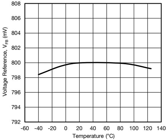
Fig. 22 - Voltage Reference vs. Junction Temperature
