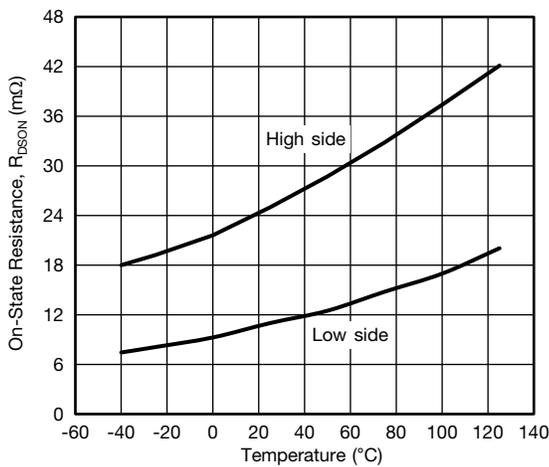
**Fig. 12 - On Resistance vs. Junction Temperature**
