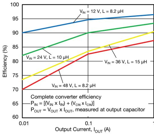
**Fig. 14 - Efficiency vs. Output Current**
