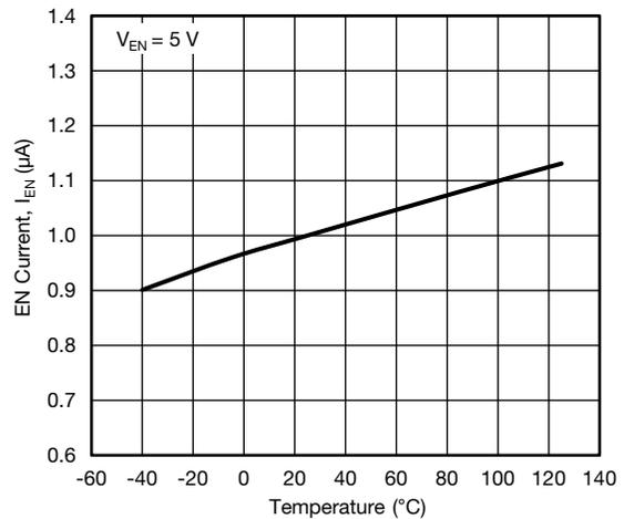
**Fig. 21 - EN Current vs. Junction Temperature**
