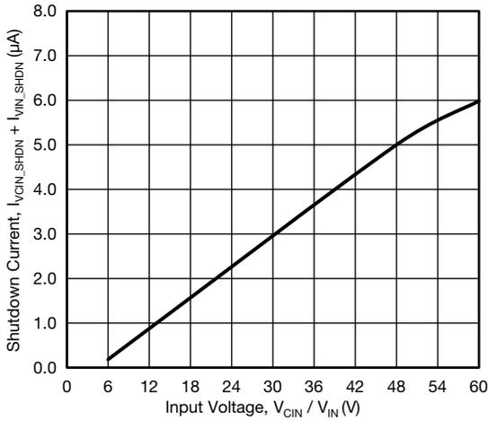
**Fig. 16 - Shutdown Current vs. Input Voltage**
