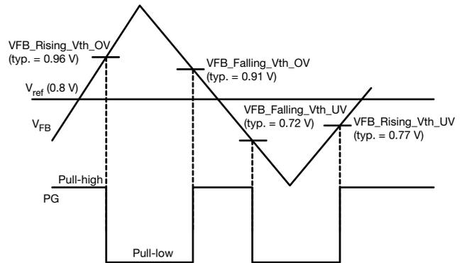
**Fig. 8 - P\_GOOD Window and Timing Diagram**
