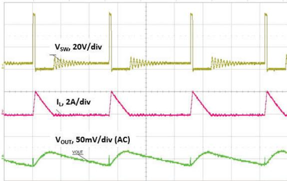
**Fig. 28 - Output Ripple 300 mA, Time = 5  $\mu$ s/div**
