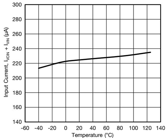
**Fig. 15 - Input Current vs. Junction Temperature**
