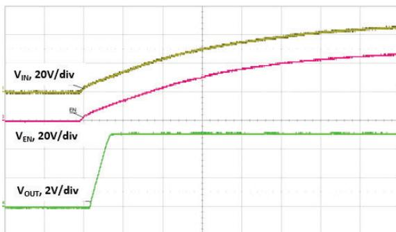
Fig. 24 - Start-Up with  $V_{IN}$ , Time = 5 ms/div
