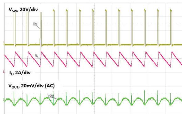
Fig. 27 - Output Ripple 2 A, Time = 5  $\mu$ s/div
