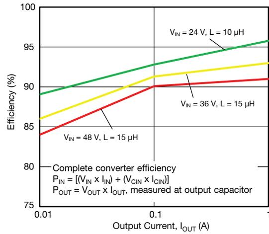
**Fig. 13 - Efficiency vs. Output Current**
