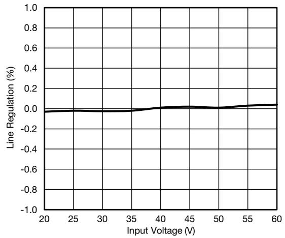
**Fig. 20 - Line Regulation,  $V_{OUT} = 12\text{ V}$**
