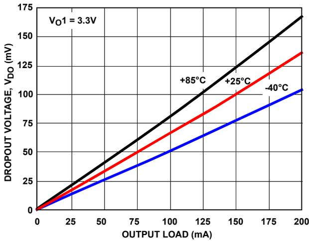
FIGURE 7. VO1 DROPOUT VOLTAGE vs LOAD CURRENT
