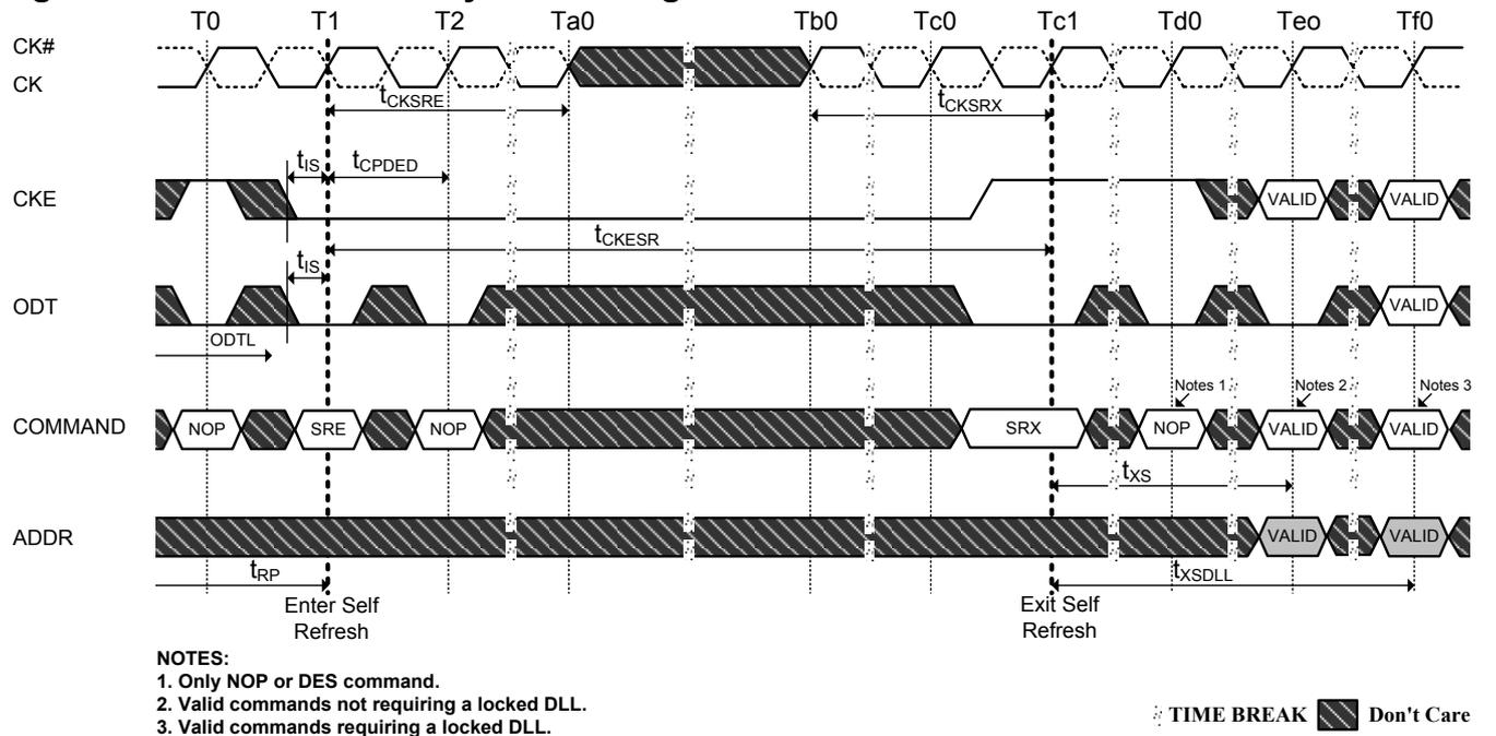
**Figure 55. Active Power-Down Entry and Exit Timing Diagram**
