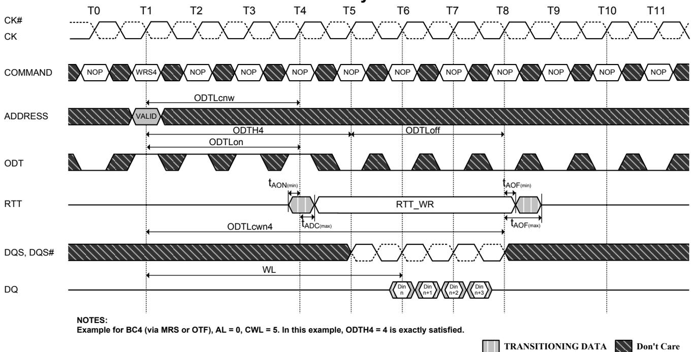
**Figure 72. Asynchronous ODT Timings on DDR3L SDRAM with fast ODT transition**
