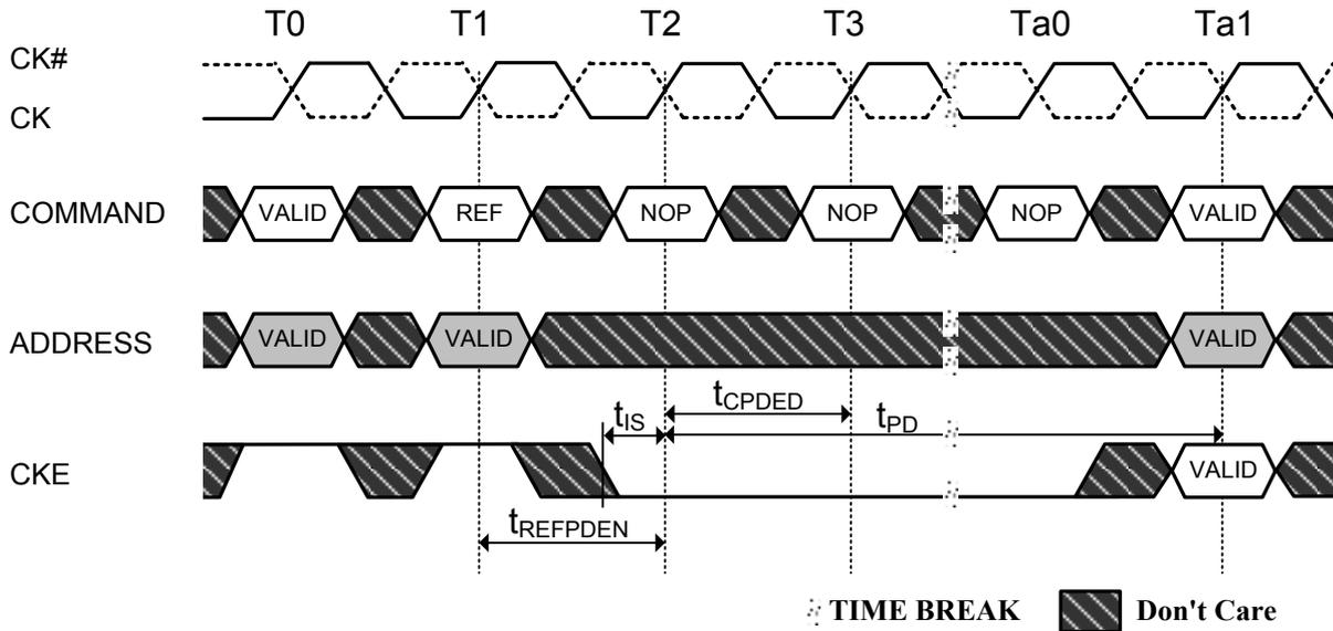
**Figure 62. Active Command to Power-Down Entry**
