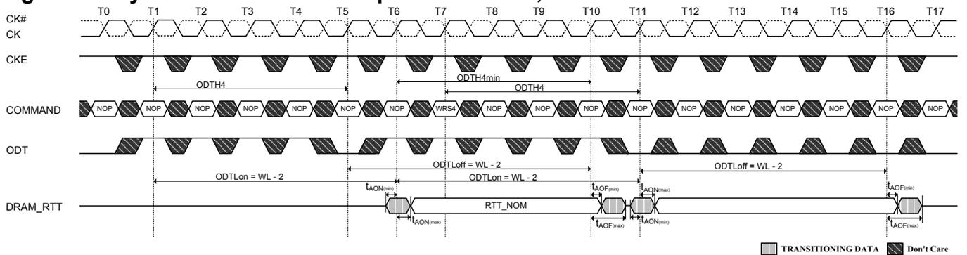
**Figure 67. Dynamic ODT Behavior with ODT being asserted before and after the write**
