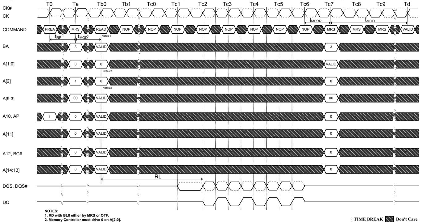
**Figure 26. MPR Readout of predefined pattern, BL8 fixed burst order, back to back readout**
