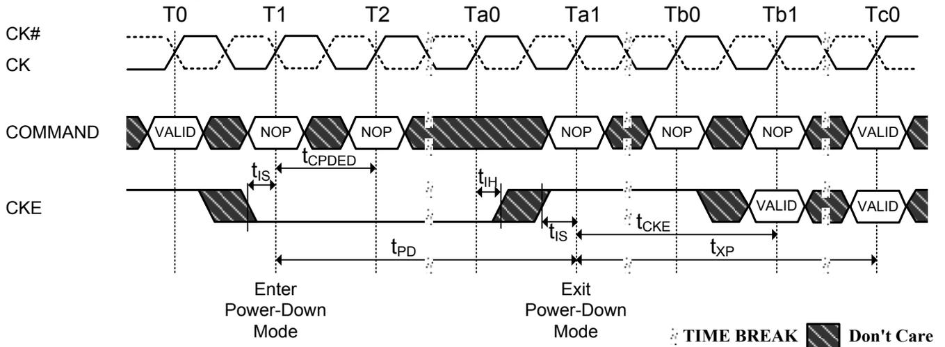
**Figure 60. Precharge Power-Down (Slow Exit Mode) Entry and Exit**
