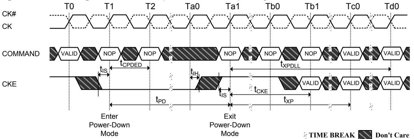
**Figure 61. Refresh Command to Power-Down Entry**
