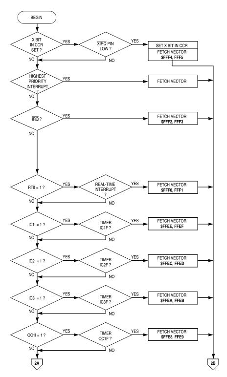
Figure 5-6. Interrupt Priority Resolution (Sheet 1 of 2)
