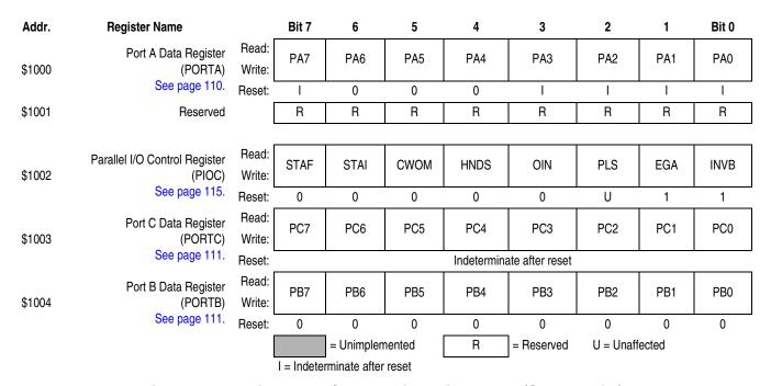
Figure 2-7. Register and Control Bit Assignments (Sheet 1 of 6)
