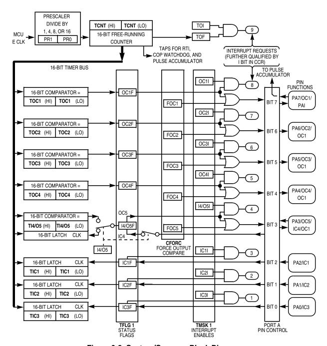
Figure 9-2. Capture/Compare Block Diagram
