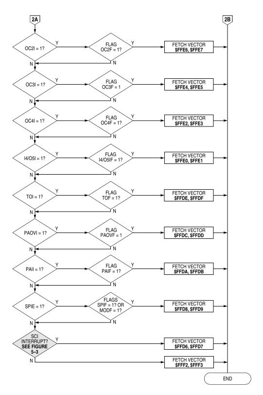
Figure 5-6. Interrupt Priority Resolution (Sheet 2 of 2)
