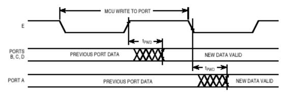
Figure 10-8. Port Write Timing Diagram
