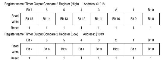
Figure 9-9. Timer Output Compare 2 Register Pair (TOC2)
