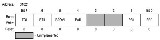
Figure 9-19. Timer Interrupt Mask 2 Register (TMSK2)
