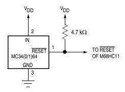
Figure 1-7. External Reset Circuit
