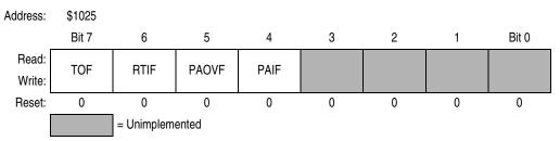
Figure 9-22. Timer Interrupt Flag 2 Register (TFLG2)
