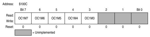
Figure 9-13. Output Compare 1 Mask Register (OC1M)
