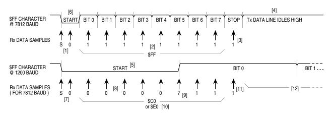
Figure 2. Automatic Detection of Baud Rate
