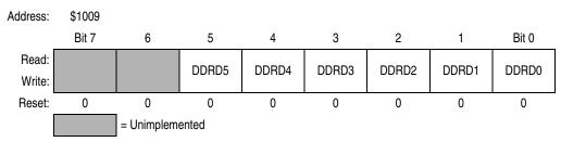
Figure 6-8. Port D Data Direction Register (DDRD)
