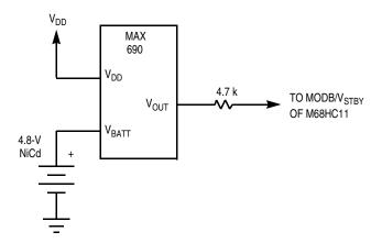
Figure 2-8. RAM Standby MODB/V<sub>STBY</sub> Connections
