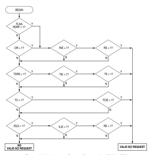
Figure 7-10. Interrupt Source Resolution Within SCI
