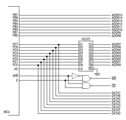
Figure 2-1. Address/Data Demultiplexing
