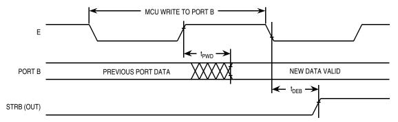
Figure 10-10. Simple Output Strobe Timing Diagram
