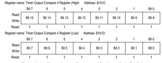
Figure 9-11. Timer Output Compare 4 Register Pair (TOC4)
