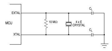
Figure 1-9. Common Parallel Resonant Crystal Connections
