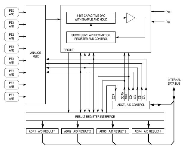
Figure 3-1. A/D Converter Block Diagram
