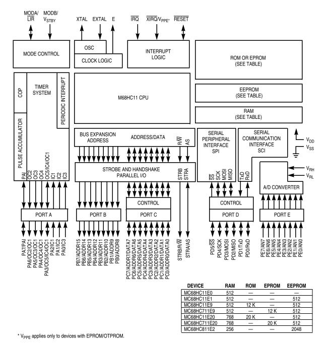
Figure 1-1. M68HC11 E-Series Block Diagram
