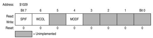
Figure 8-4. Serial Peripheral Status Register (SPSR)
