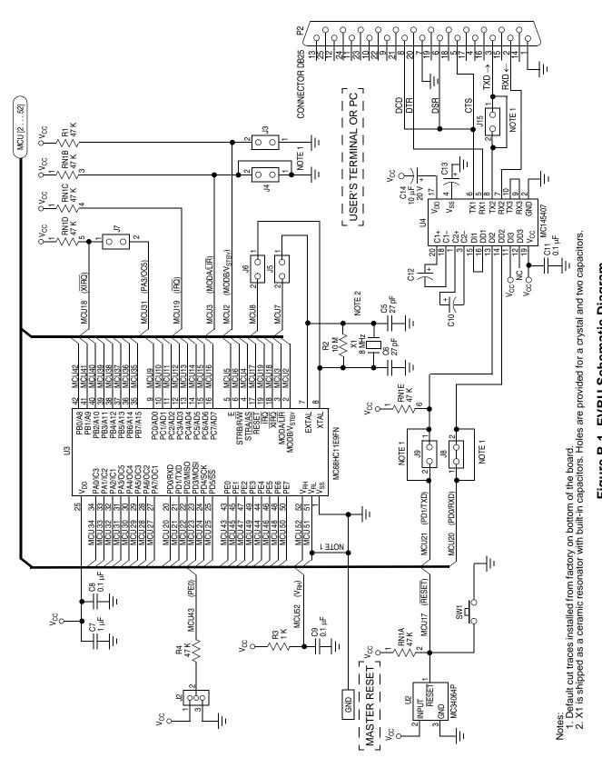
Figure B-1. EVBU Schematic Diagram
