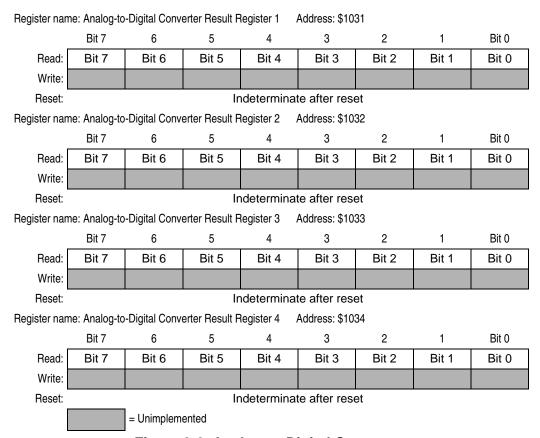
Figure 3-6. Analog-to-Digital Converter Result Registers (ADR1–ADR4)
