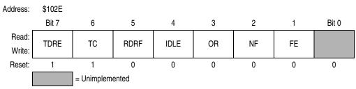
Figure 7-6. Serial Communications Status Register (SCSR)
