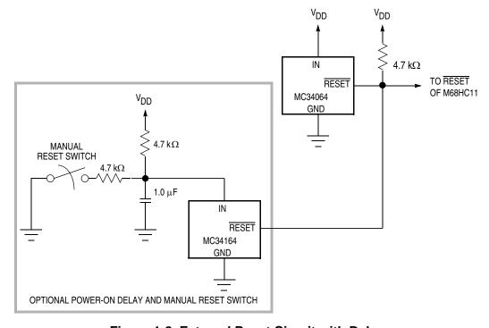
Figure 1-8. External Reset Circuit with Delay
