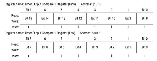
Figure 9-8. Timer Output Compare 1 Register Pair (TOC1)
