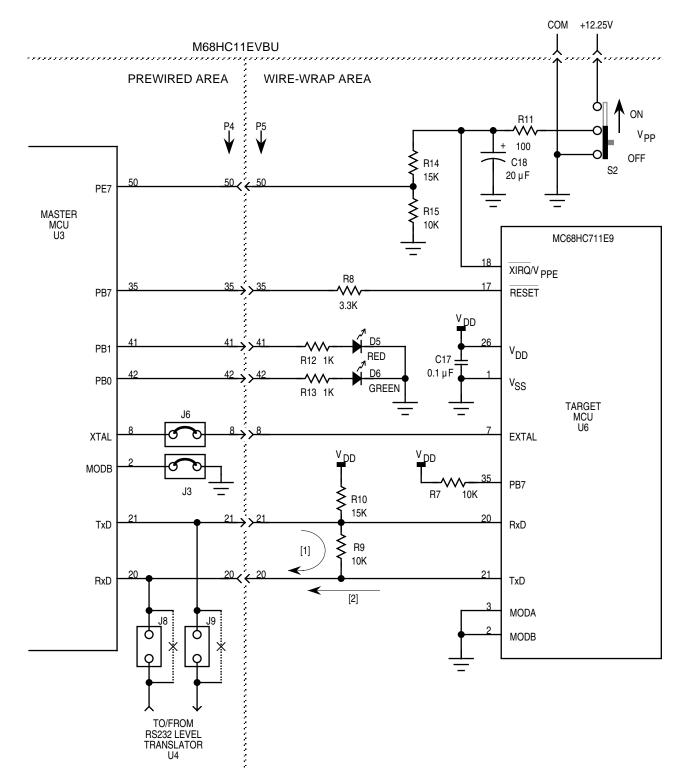
Figure 6. MCU-to-MCU EPROM Duplicator Schematic
