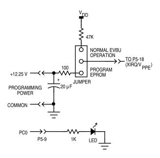
Figure 8. PC-to-MCU Programming Circuit
