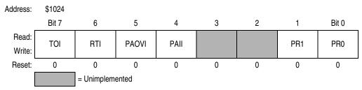
Figure 9-21. Timer Interrupt Mask 2 Register (TMSK2)
