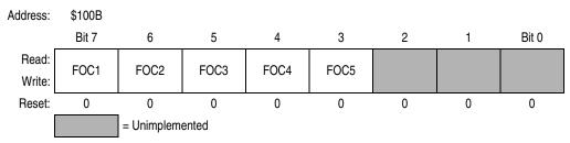
Figure 9-12. Timer Compare Force Register (CFORC)
