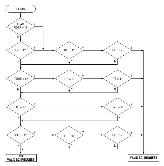
Figure 5-7. Interrupt Source Resolution Within SCI
