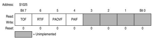
Figure 9-20. Timer Interrupt Flag 2 Register (TFLG2)
