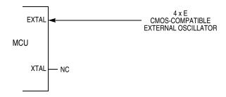
Figure 1-10. External Oscillator Connections
