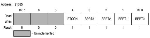
Figure 2-16. Block Protect Register (BPROT)
