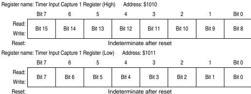
Figure 9-4. Timer Input Capture 1 Register Pair (TIC1)
