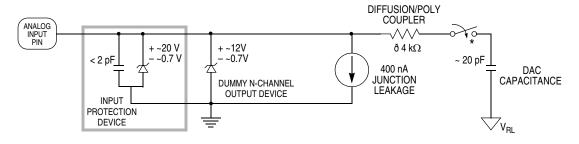
\* THIS ANALOG SWITCH IS CLOSED ONLY DURING THE 12-CYCLE SAMPLE TIME.
