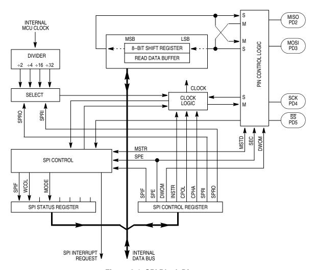
Figure 8-1. SPI Block Diagram
