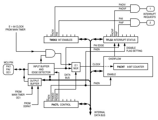
Figure 9-24. Pulse Accumulator
