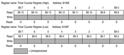
Figure 9-15. Timer Counter Register (TCNT)
