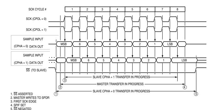
Figure 8-2. SPI Transfer Format
