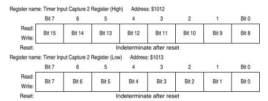
Figure 9-5. Timer Input Capture 2 Register Pair (TIC2)
