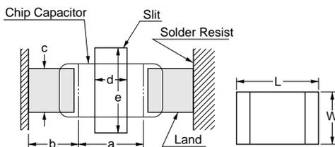
Preparing slit help flux cleaning and resin coating on the back of the capacitor.
