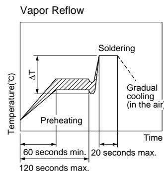
[Allowable Soldering Temperature and Time]
