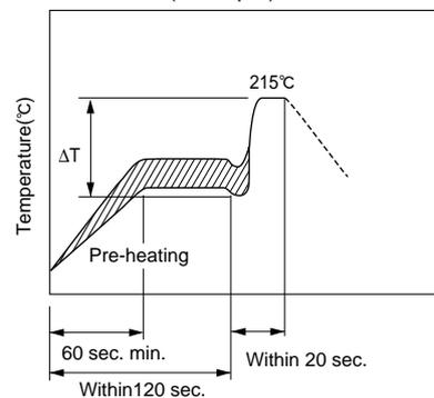
Flow Soldering Conditions (Example)
