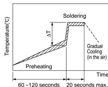
[Allowable Time and Temperature for Making Corrections with a Soldering Iron]
