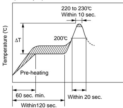
Vapor Reflow Soldering (VPS) Conditions (Example)
