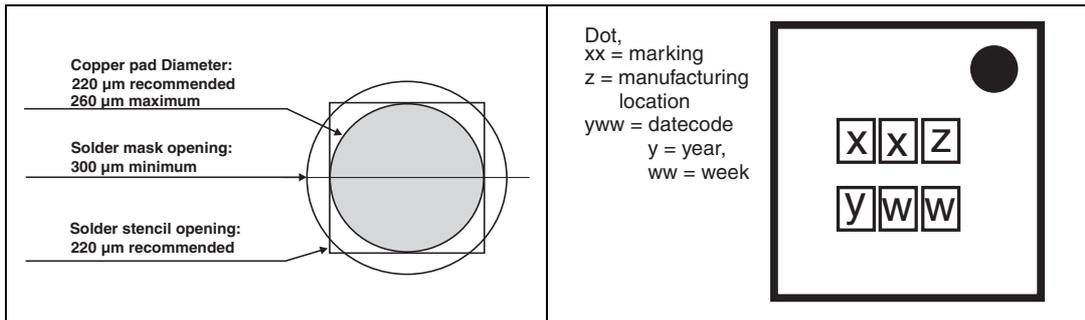
**Note:** Product marking may be rotated by  $90^\circ$  for assembly plant differentiation. In no case should this product marking be used to orient the component for its placement on a PCB. Only pin 1 mark is to be used for this purpose.
