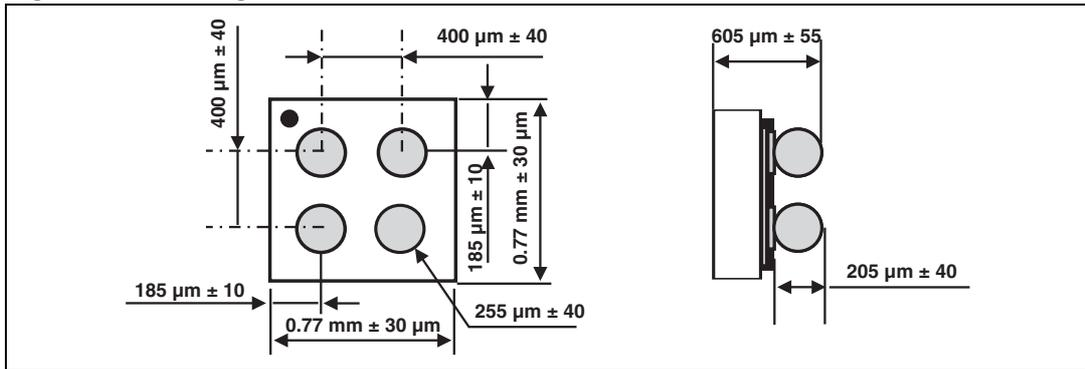
**Figure 18. Foot print recommendations**      **Figure 19. Marking**
