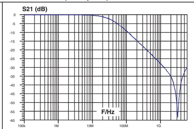
Figure 14. ESD response to IEC 61000-4-2 (+8 kV contact discharge)
