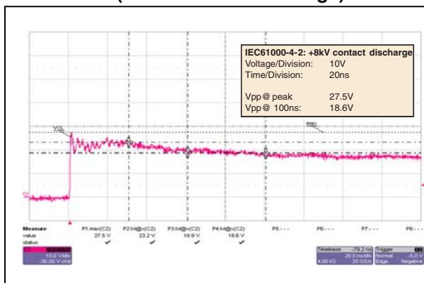
Figure 15. ESD response to IEC 61000-4-2 (-8 kV contact discharge)
