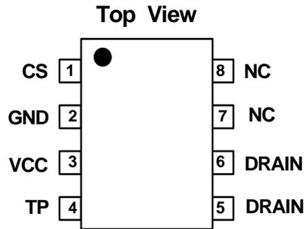
**Figure 2. Pin Assignments**
