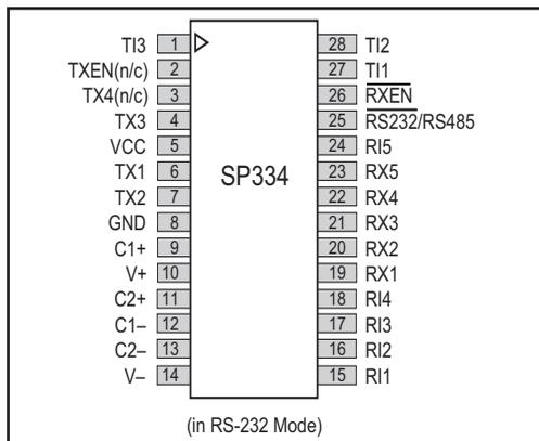
Figure 11. SP334 Pinout
