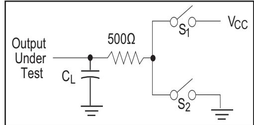
Figure 4. Driver Timing Test Load #2 Circuit
