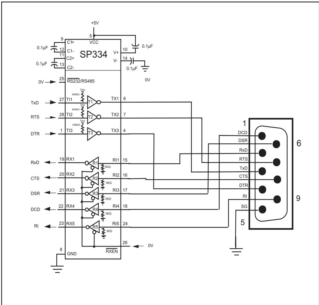
Figure 18. SP334 Configuration to a DB-9 Serial Port
