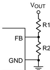
Figure 1. Setting  $V_{OUT}$  with a Voltage Divider
