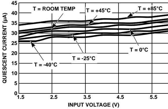
FIGURE 1. QUIESCENT CURRENT vs INPUT VOLTAGE (V<sub>OUT</sub> = 0.9V)
