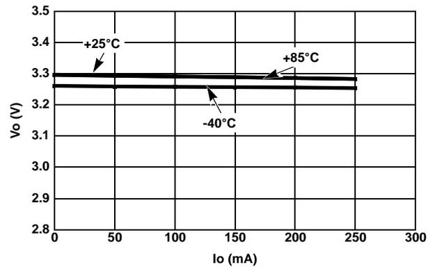
FIGURE 6. LOAD REGULATION vs TEMPERATURE (V<sub>OUT</sub> = 3.3V)
