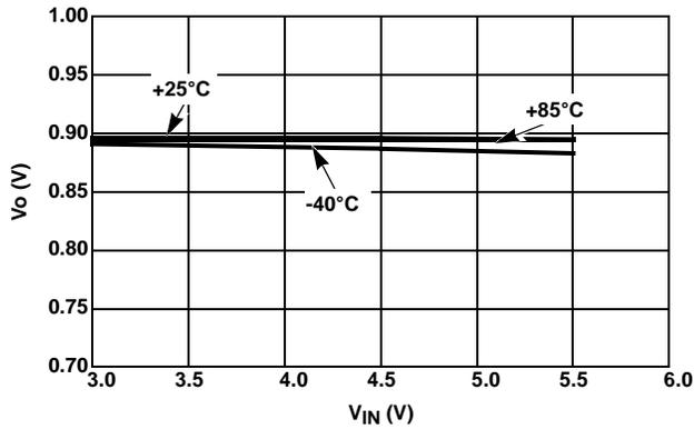
FIGURE 9. LINE REGULATION vs TEMPERATURE
