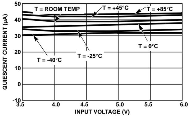
FIGURE 3. QUIESCENT CURRENT vs INPUT VOLTAGE (V<sub>OUT</sub> = 3.3V)
