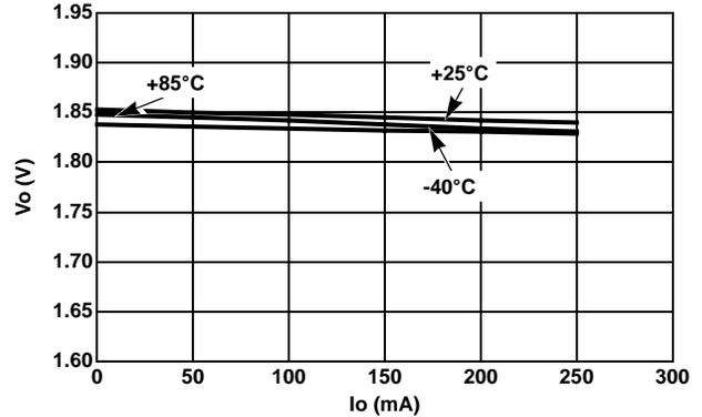
FIGURE 4. LOAD REGULATION vs TEMPERATURE (V<sub>OUT</sub> = 1.85V)
