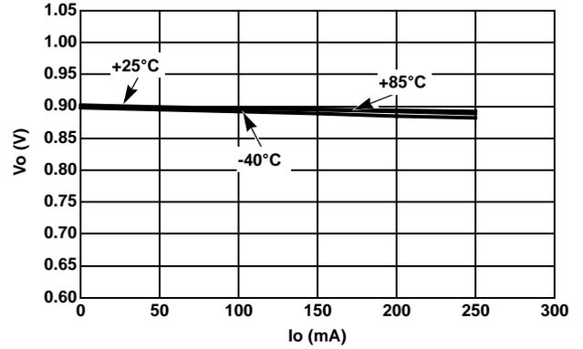
FIGURE 8. LOAD REGULATION vs TEMPERATURE
