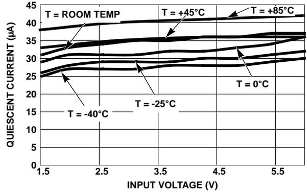
FIGURE 2. QUIESCENT CURRENT vs INPUT VOLTAGE (V<sub>OUT</sub> = 1.85V)
