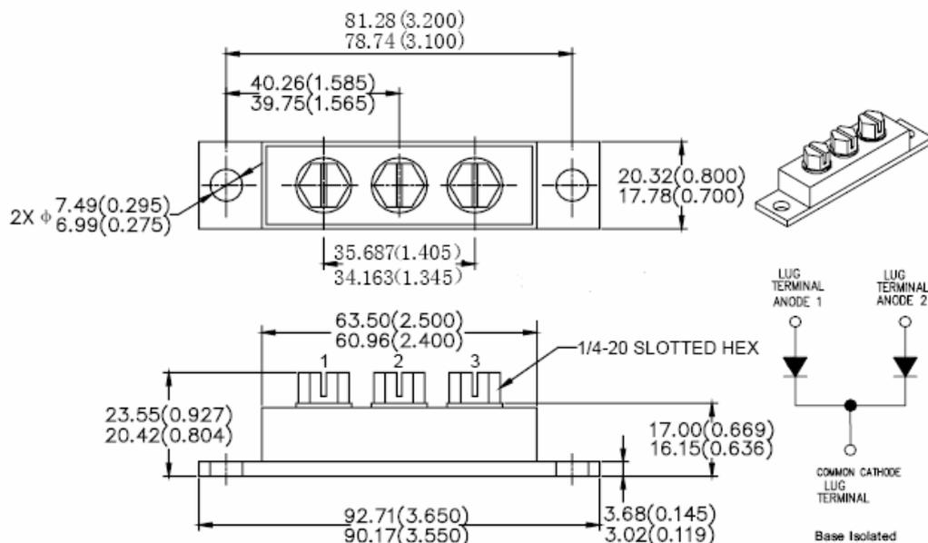
Please Note: Anode 1 = Terminal 1; Anode 2 = Terminal 3; Common Cathode = Terminal 2
