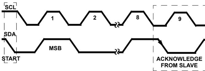
FIGURE 17. ACKNOWLEDGE ON THE I<sup>2</sup>C BUS
