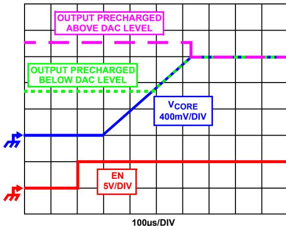
FIGURE 12. SOFT-START WAVEFORMS FOR ISL6324-BASED MULTIPHASE CONVERTER
