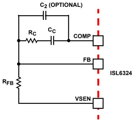
FIGURE 23. COMPENSATION CONFIGURATION FOR LOAD-LINE REGULATED ISL6324 CIRCUIT
