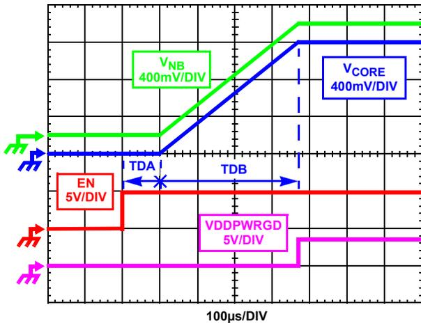
FIGURE 11. SOFT-START WAVEFORMS
