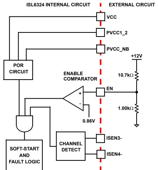
FIGURE 10. POWER SEQUENCING USING THRESHOLD-SENSITIVE ENABLE (EN)
