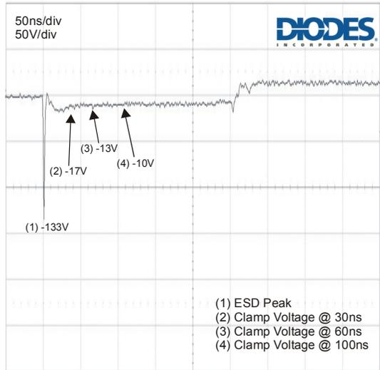
Figure 12 ESD Response to IEC 6100-4-2 (-15kV Contact Discharge)
