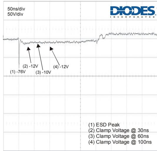
Figure 10 ESD Response to IEC 6100-4-2 (-8kV Contact Discharge)
