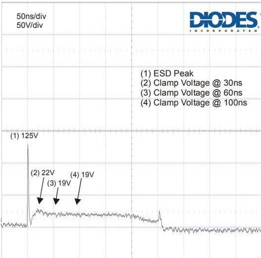
Figure 11 ESD Response to IEC 6100-4-2 (+15kV Contact Discharge)
