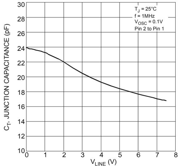
Figure 8 Junction Capacitance vs. Reverse Voltage (Typical Values)
