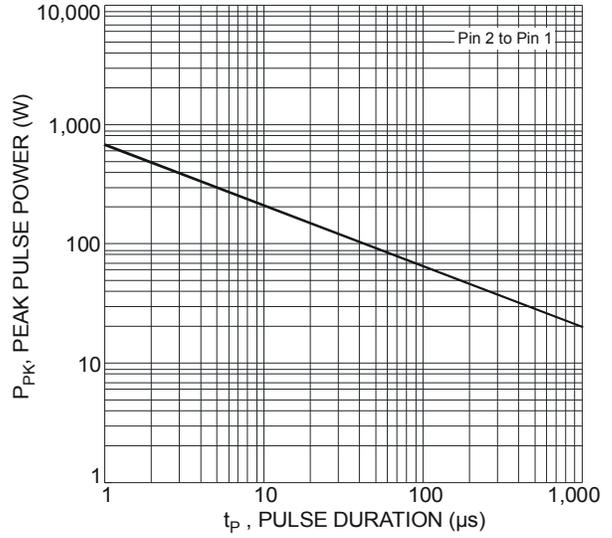
Figure 4 Peak Pulse Power vs. Pulse Duration
