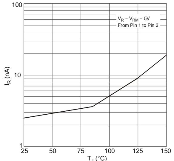
Figure 2 Leakage Current vs. Junction Temperature (Typical Values)
