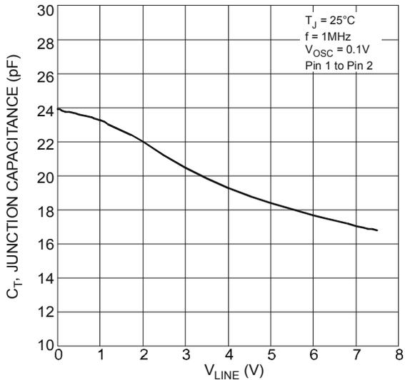
Figure 7 Junction Capacitance vs. Reverse Voltage (Typical Values)
