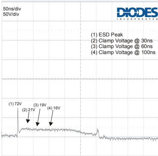
Figure 9 ESD Response to IEC 6100-4-2 (+8kV Contact Discharge)
