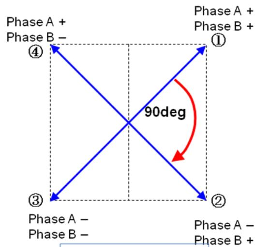
Figure 11. Motor electric angle (Full Step Drive)
