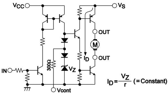
As shown in the left diagram, the Vcont pin outputs the voltage of the band gap Zener  $V_Z + V_F (= 1.93V)$ . In normal use, this pin is left open. The drive current  $I_D$  is varied by the Vcont voltage. However, because the band gap Zener is shared, it functions as a bridge. The motor can stop by making vcont terminal GND in emergency.
