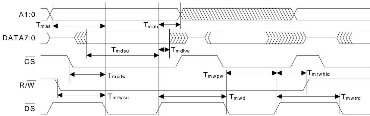
**Figure 6. Motorola® Parallel Host Mode Write Cycle**
