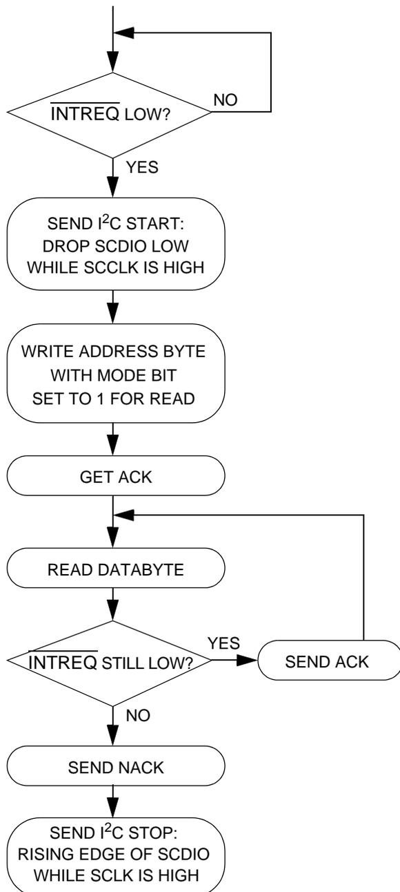
**Figure 23. I<sup>2</sup>C® Read Flow Diagram**
