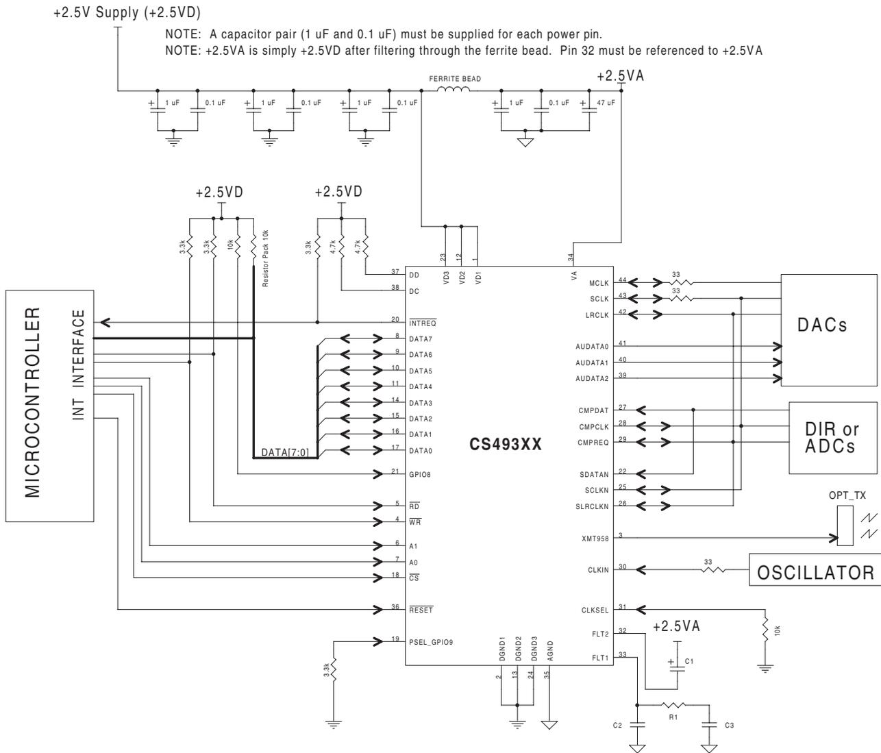
Figure 17. Intel® Parallel Control Mode
