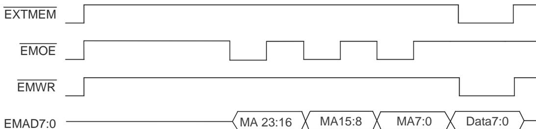
**Figure 32. External Memory Write (16-bit address)**
