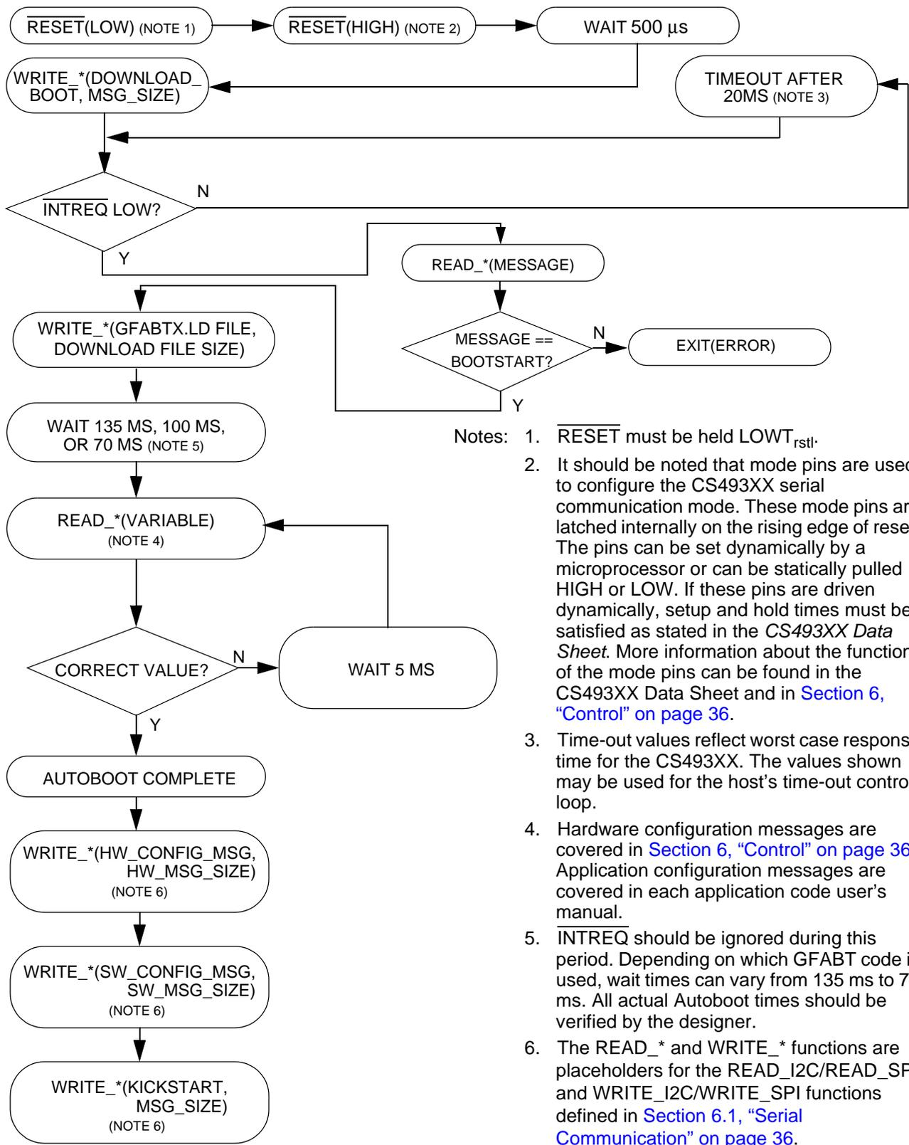
**Figure 38. Fast Autoboot Sequence Using GFABT Codes**
