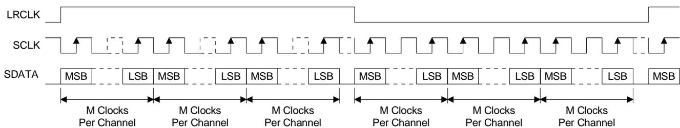
**Figure 45. Multichannel Format**
