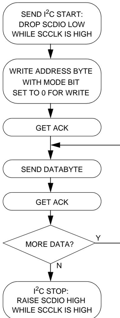
**Figure 22. I<sup>2</sup>C® Write Flow Diagram**
