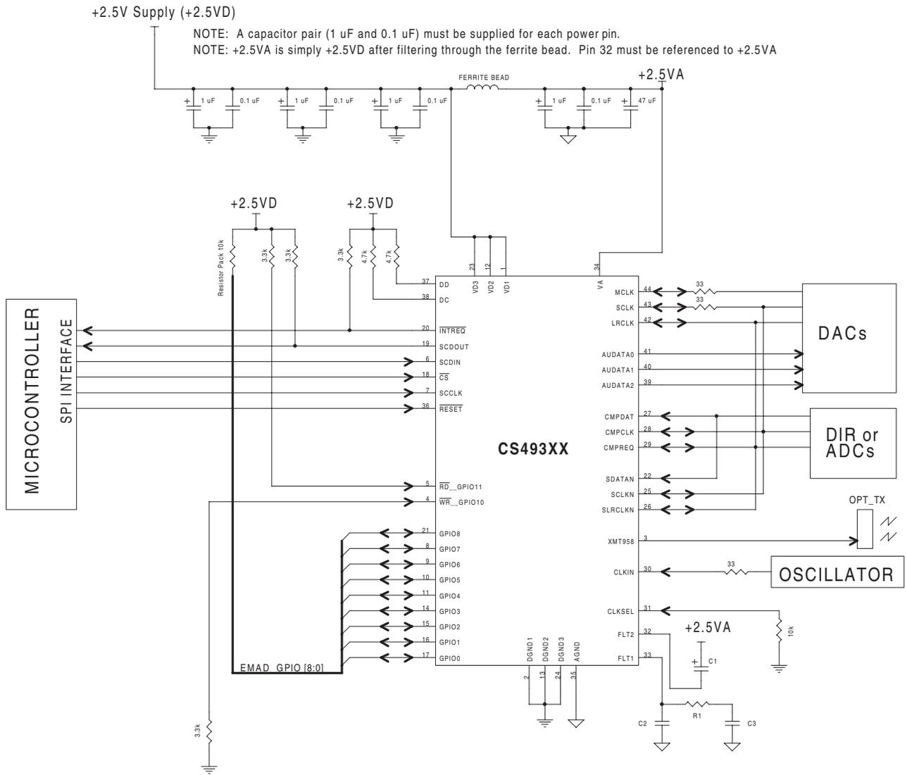
Figure 15. SPI Control
