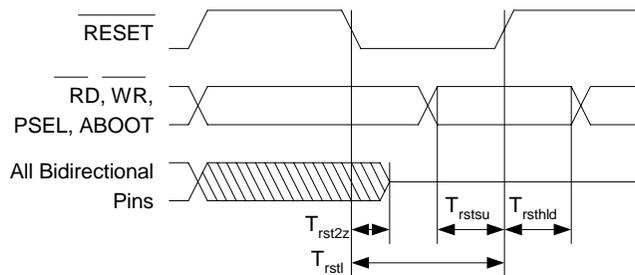
**Figure 1. RESET Timing**
