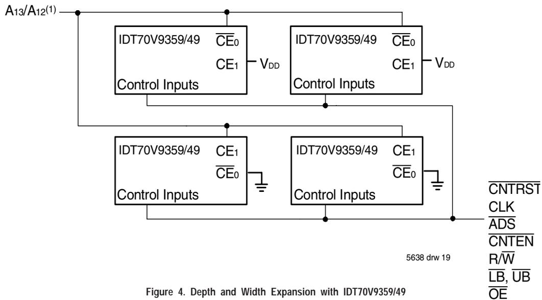
Figure 4. Depth and Width Expansion with IDT70V9359/49
