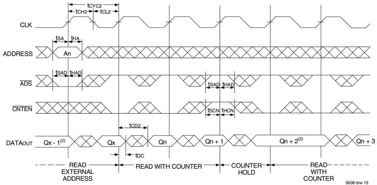
Timing Waveform of Flow-Through Read with Address Counter Advance<sup>(1)</sup>
