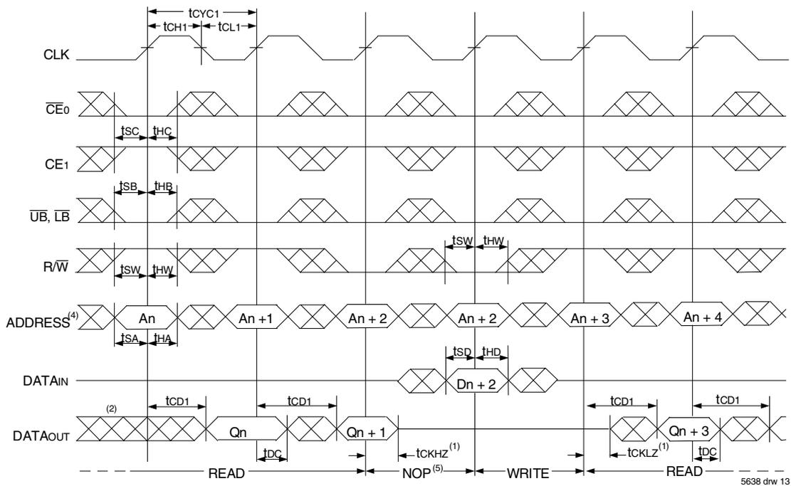
Timing Waveform of Flow-Through Read-to-Write-to-Read ( $\overline{OE}$  Controlled)<sup>(3)</sup>
