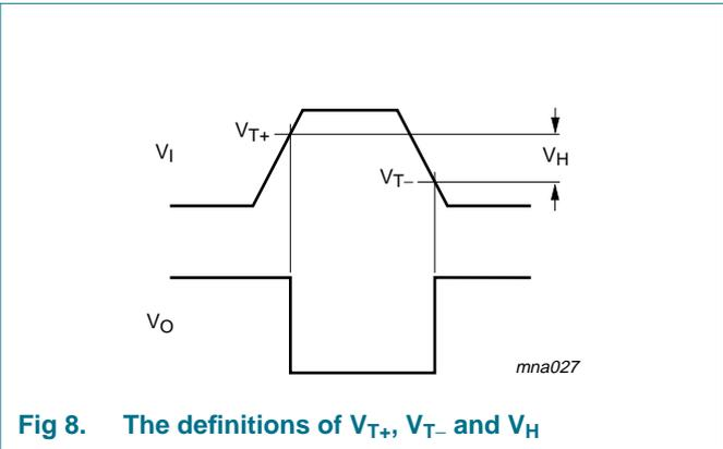
**Fig 8. The definitions of  $V_{T+}$ ,  $V_{T-}$  and  $V_H$**
