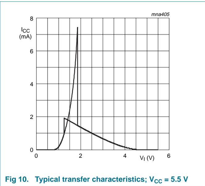
**Fig 10. Typical transfer characteristics;  $V_{CC} = 5.5$  V**
