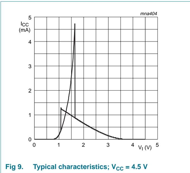
**Fig 9. Typical characteristics;  $V_{CC} = 4.5$  V**
