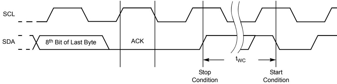
**Nonvolatile Write Cycle Timing**
