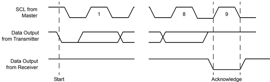
Figure 9. Byte Write Sequence
