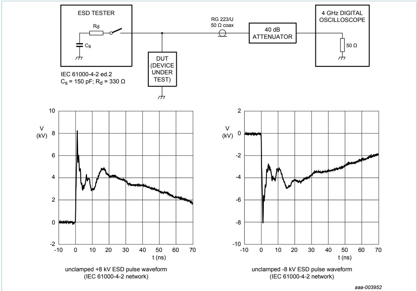
Fig. 11. ESD clamping test setup and waveforms
