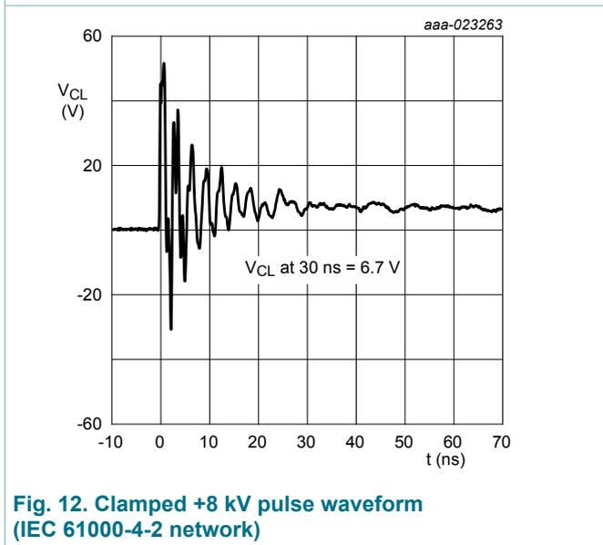
Fig. 12. Clamped +8 kV pulse waveform (IEC 61000-4-2 network)
