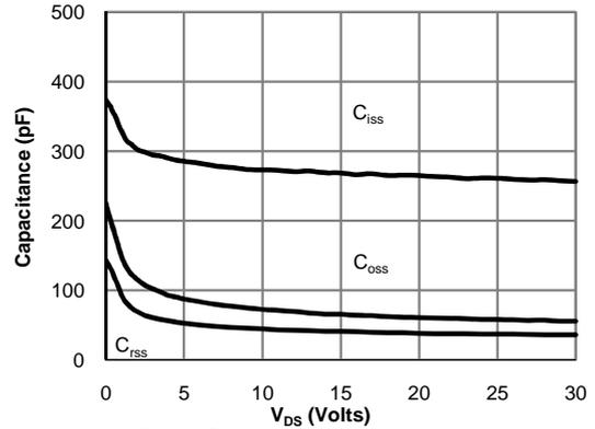
Figure 8: Capacitance Characteristics
