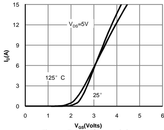
Figure 2: Transfer Characteristics
