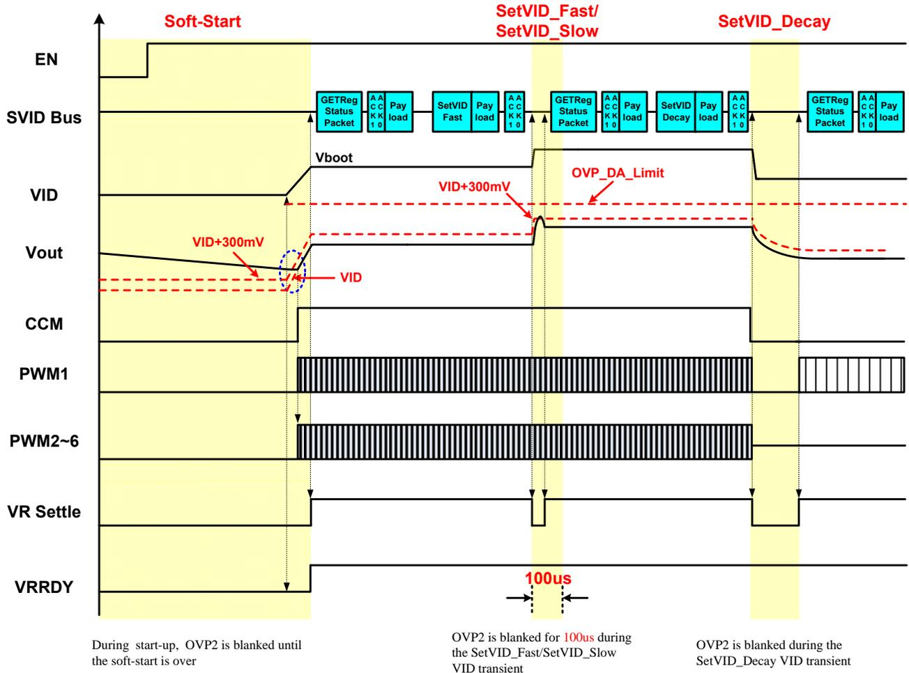
FIGURE 12. OVP Protection Blanking Conditions
