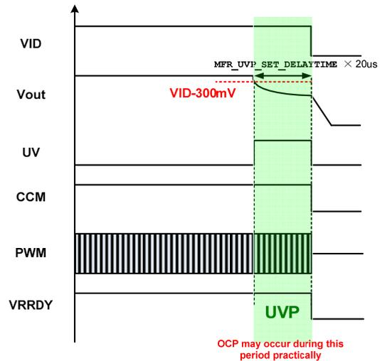
FIGURE 16. Under-Voltage Protection
