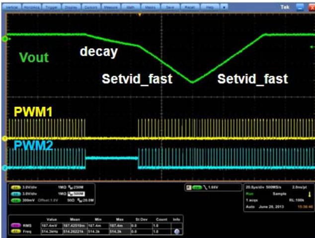
FIGURE 10(a). Decay (Interrupted) → SetVID\_Fast (Interrupted) → SetVID\_Fast (Finished)
