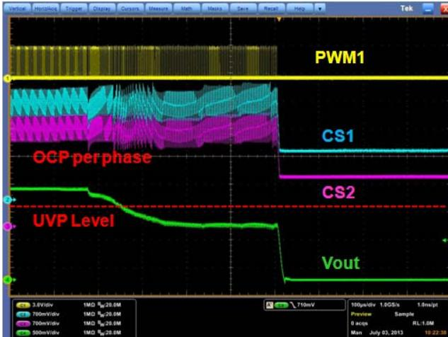
**FIGURE17. UVP Triggered when Per-Phase Current is Limited**
