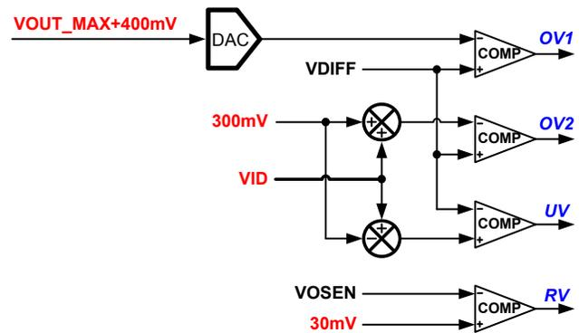
**FIGURE 11. OV, UV, and RV Signal Generation**
