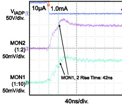
$I_{APD} = 2mA$ ,  $V_{IN} = 2.7V$
