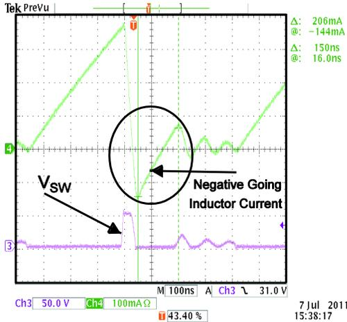
Due to the applied high-output voltage on the switch node combined with the  $C_{DS}$  capacitive coupling of the MP3430 FET, a significant reverse current flows through the inductor during the  $D_3$  period.
