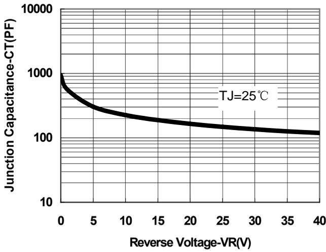
Fig.1-Typical Junction Capacitance
